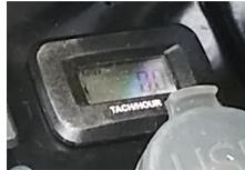
Reads current motor speed or total hours of operation. Push button toggles display.
